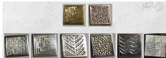
Figure 3. Experiments Comparing Hand Engraving Techniques Using Hand Tools And Rotary Tools On 20mmx20mm Silver Plate
