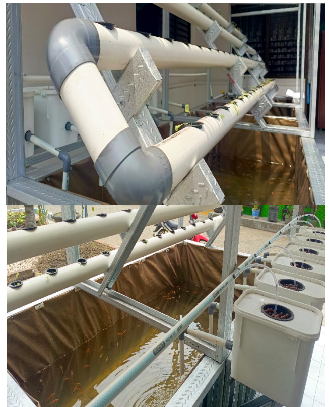
Figure 3. Aquaponic with recirculating aquaculture system
