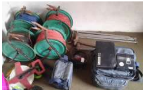
Gambar 2. Set Peralatan Geolistrik
