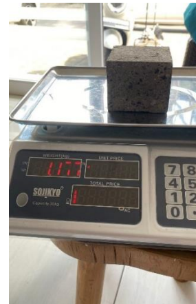
Gambar 1.12 Berat Kering Paving Block 3
