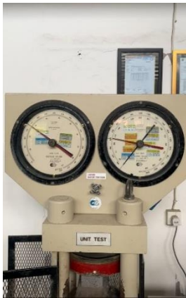
Gambar 1.9 Uji Kuat Tekan Paving Block 3
