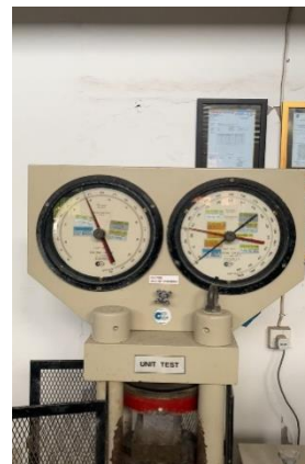
Gambar 1.8 Uji Kuat Tekan Paving Block 2
