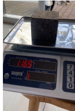
Gambar 1.10 Berat Kering Paving Block 1
