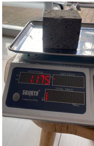
Gambar 1.11 Berat Kering Paving Block 2
