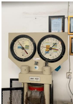
Gambar 1.7 Uji Kuat Tekan Paving Block 1
